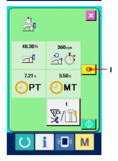
When CLEAR button C (J) is pressed in the clear confirmation screen, the counted value is cleared.
