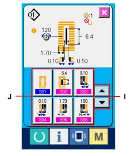
※ Now, input has been completed. However, for the continuous stitching, enter all data within the range of the presser size. When the data is outside the range, error is displayed. Be sure to correctly input the presser size. →Refer to 2-8. INPUTTING THE PRESSER TYPE,p.56.
